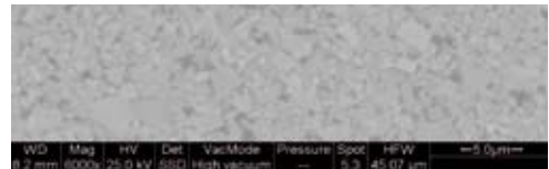
Fig. 3.6: Micrograph showing etched surface of tungsten carbide
