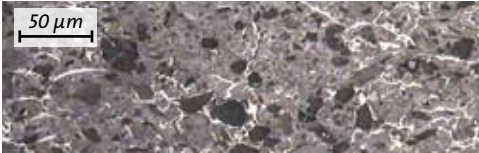
Fig. 3.1: Micrograph showing the material structure of antimony-impregnated carbon graphite
