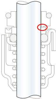
Small amounts of hard particles on the seal faces result in increased wear, especially when using hard/soft seal face material pairings. In such cases, small, hard particles might be squeezed into the soft seal ring from where they act as a grinding tool on the hard seal ring.
