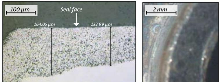
*Fig. 5.9: Selective corrosion in cemented tungsten carbide. The metallic binder phase is corroded resulting in reduced wear resistance*
