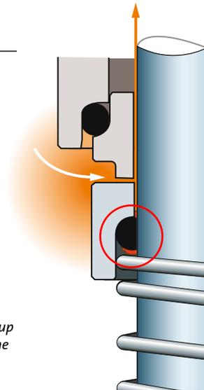
*Fig. 5.5: Sketch of seal hang-up due to blocking of the axial movement of the dynamic O-ring*
