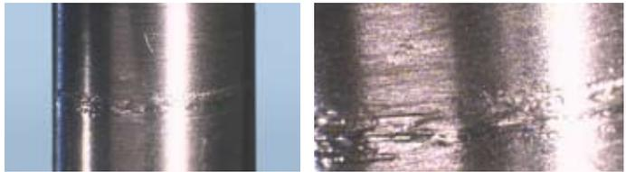
Fig. 5.18: Corrosion on shaft below dynamic O-ring caused by axial movement of the shaft
