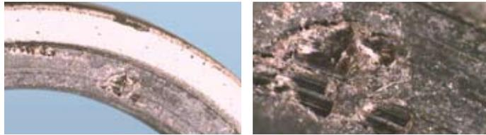
Fig. 5.6: Deposits on carbon graphite seal face
