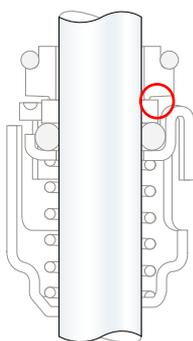
mechanical properties, including decrease in wear resistance. When the metallic binder phase disappears, the surface becomes matted. The selective corrosion of the binder phase may induce stresses, leading to cracks in the seal rings. See fig. 5.9.
