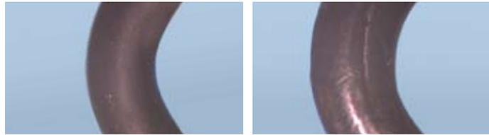
*Fig. 5.8: A fresh EPDM O-ring (left) and a swollen EPDM O-ring (right) exposed to water containing mineral oil*
