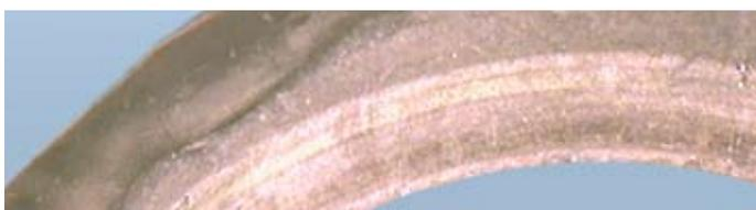
*Fig. 5.10: Corrosion of the binder phase followed by severe erosion on a tungsten carbide seal ring with cobalt binder phase*
